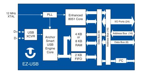
The Anchor Chips EZ-USB<sup>TM</sup> family (AN21XX/AN23XX) provides significant improvements over other USB architectures including an enhanced 8051 core, 4 or 8 Kbytes of RAM, an intelligent USB core, and high-performance I/O ports. The family includes 16 different products to accommodate the needs of different systems.
